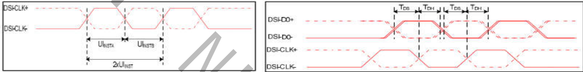
Figure 4 DSI clock channel timing
